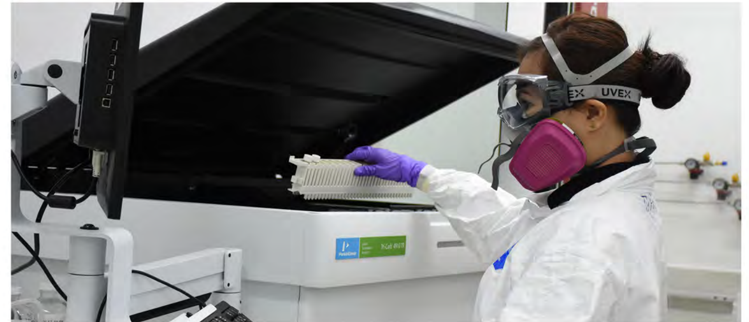
Dianne Dasmariñas, Laguna Water Laboratory Analyst, demonstrates how to load sample for Alpha-Beta Radioactivity Determination equipment.
